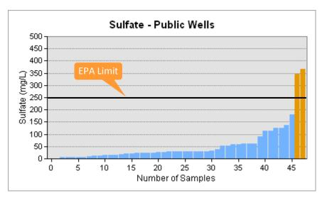
guideline is indicated by a black horizontal line at 250 mg/L. The graphs show that only a few sulfate values are higher than the EPA standard; one is extremely high and extends beyond the top of the graph.
