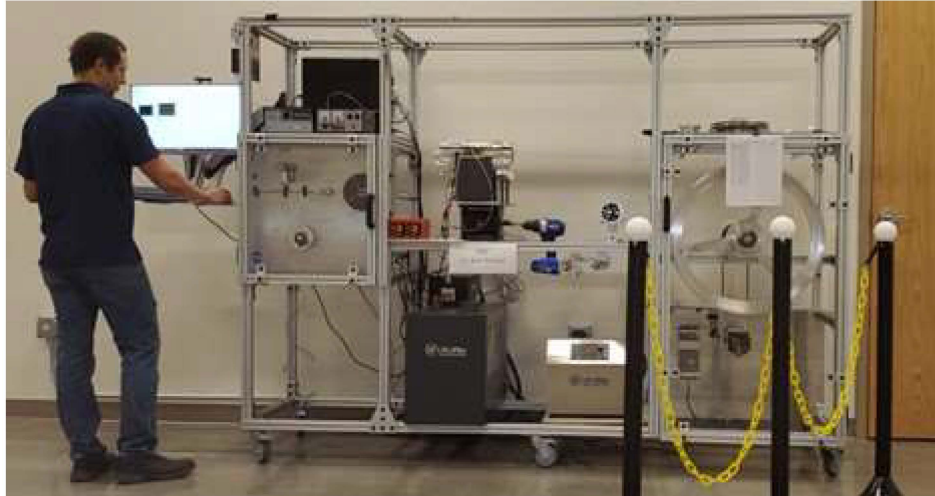
Dr. Bruno operates the in-line stress-annealing system at South Dakota Mines to tune the magnetic properties of Fe-1.5Nb-1.5W-1Cu-15.5Si-7B at.% planar-flow-cast ribbon.
