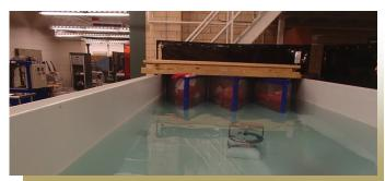
The ME department recently funded and installed a wave tank in the Integrated Laboratory to support our research on wave energy conversion. The tank is 17 ft long, 7 ft wide, and 4 ft deep, and is made of steel. Seven wave makers working on the 'oscillating water column' principle are to be installed at one end of the tank. The first of the wave maker units is already operational and can be programmed to produce
