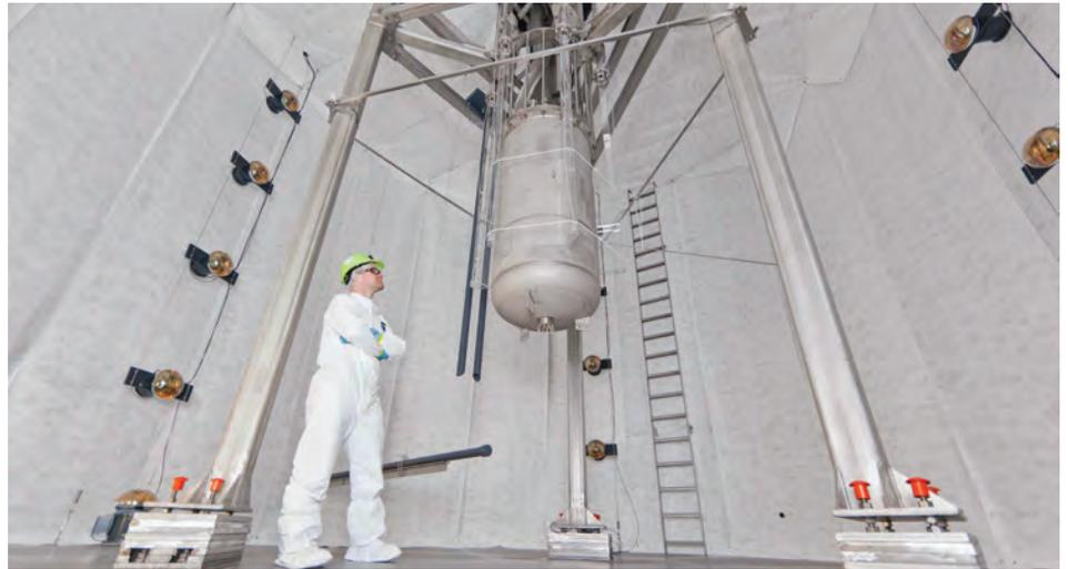
*The Large Underground Xenon (LUX)-Zeplin, or LZ, experiment at the Sanford lab is among the new projects in the search for elusive dark matter. LZ, the 7-ton version of LUX, will have a factor of 1,000 times more sensitivity.*
