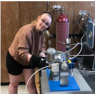
Madison Betts (MS started in Fall 2022), is preparing an experiment to be loaded in cold-seal pressure vessel. Experiments are testing the role of thermophilic bacteria on carbonate mineralization in basalt (NSF CBET Funding).
