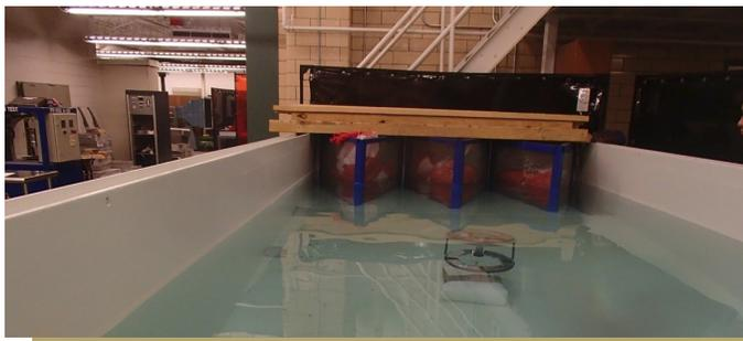
The ME department recently funded and installed a wave tank in the Integrated Laboratory to support our research on wave energy conversion. The tank is 17 ft long, 7 ft wide, and 4 ft deep, and is made of steel. Seven wave makers working on the ‘oscillating water column’ principle are to be installed at one end of the tank. The first of the wave maker units is already operational and can be programmed to produce
