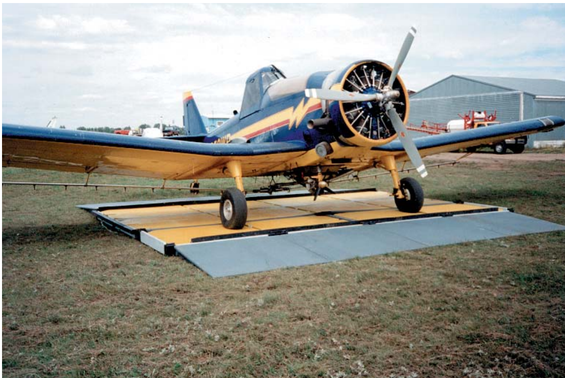
The aerial spray applicator's model of the Octa-Flex Environmental Systems containment pad developed as part of a USDA SBIR Phase II project.
