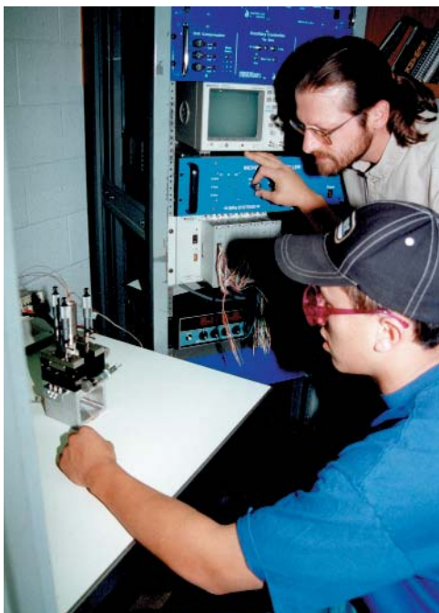
Lonnie Wright operates the interfacial force microscope to study the nano-mechanical properties of a fiberglass epoxy composite under the direction of Dr. Robb Winter, R.L. Sandvig Professor of Chemical Engineering.
